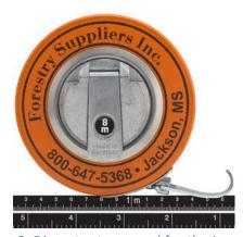
Figure 2: Diameter tape used for the inventory
